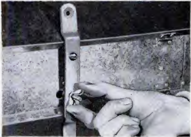
Leg which supports oven is made removable by means of horizontal keyhole slot which disengages screw
